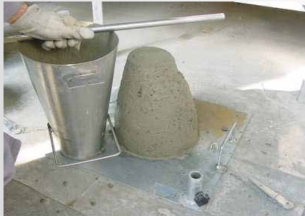
Slump S2 – 50-90mm
