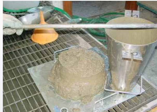
Slump S3 – 100-150mm
