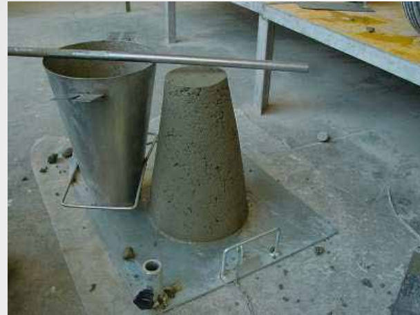
Slump S1 – 0-40mm
