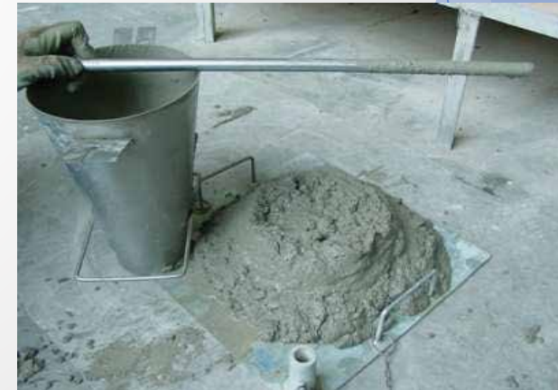
Slump S4 – 160-210mm
