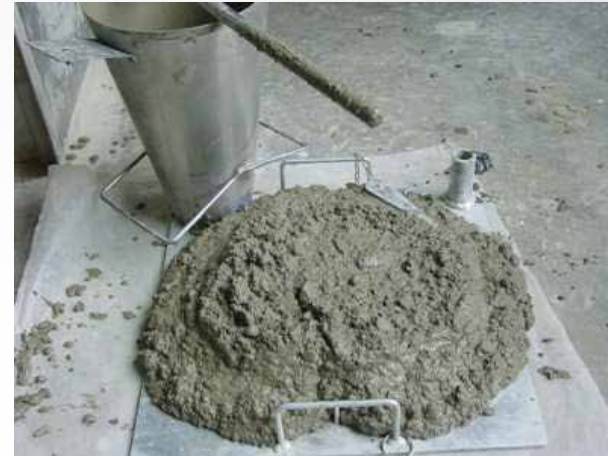
Slump S5 – > 220mm
